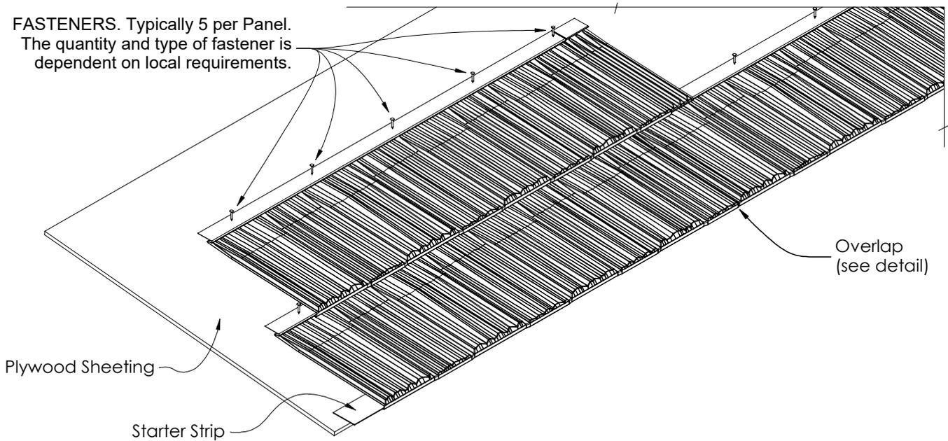
**Figure 11.2 Fastening Detail**
