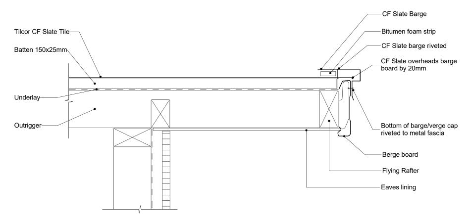
\* Barge board must not project higher than the top of tile batten
