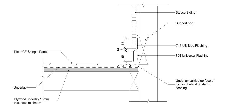
CF Shingle Side Wall Parallel Flashing with Solid Sheathing
