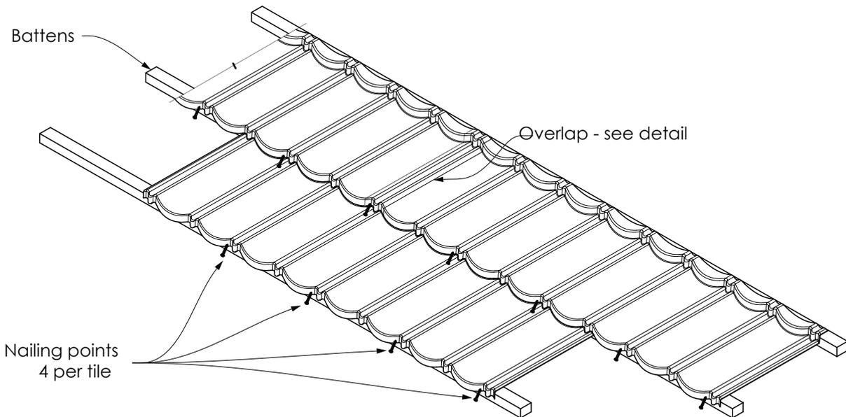
Figure 1.2 Nailing Detail
