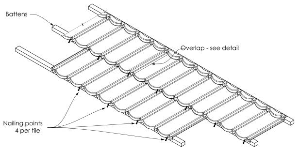
Figure 1.2 Nailing Detail
