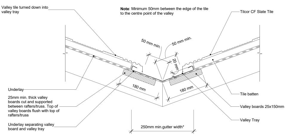
**Note**:\*Minimum width of valley tray may reduce to 160mm providing roof catchment area is 16m² or less
