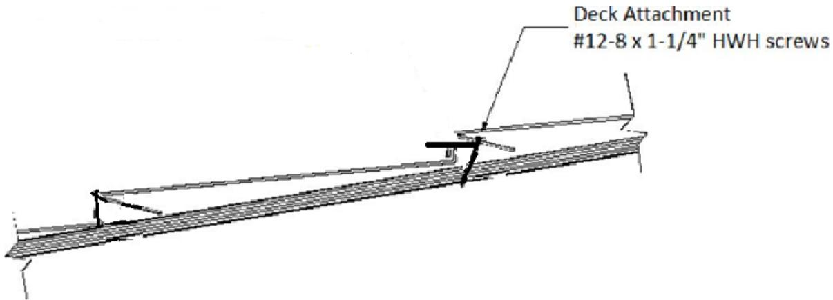
**DIRECT-TO-DECK FASTENED DETAIL**
