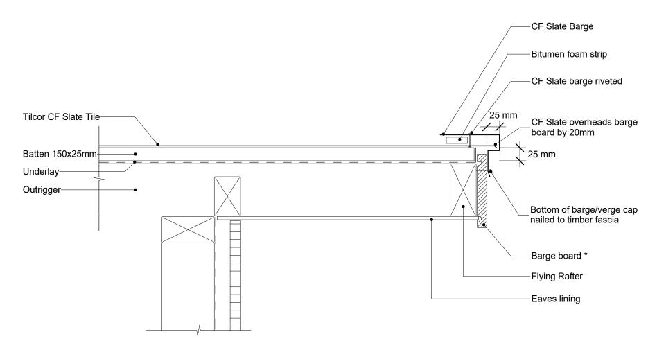
\* Barge board must not project higher than the top of tile batten
