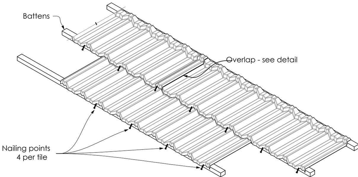
Figure 4.2 Nailing Detail
