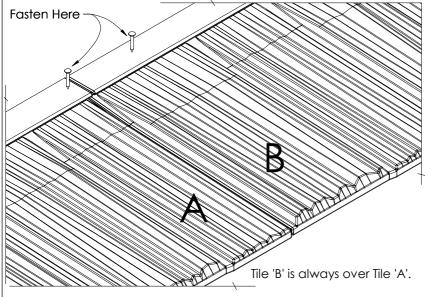
Figure 11.4 Side Lap Detail
