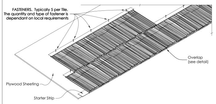
Figure 11.2 Fastening Detail
