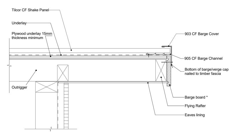
\* Barge board must not project higher than the top of plywood sheet
