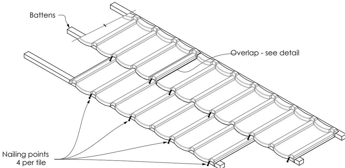
Figure 6.2 Nailing Detail
